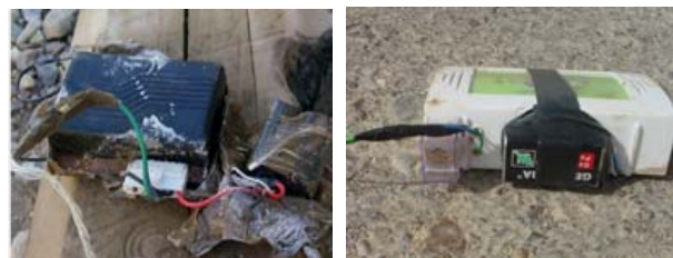
RC Unit from Car Alarm
