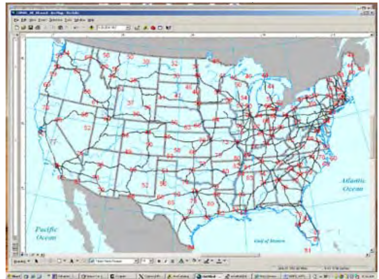
By sending the GetFeature request, a GIS application receives NDFD data for 194 points located in cities across the United States.
